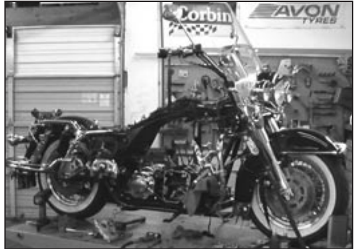
Here is an '03 Road King that just got a 103" Screamin Eagle Kit and is now getting Gear Driven Oil Pump and Cam Assembly
