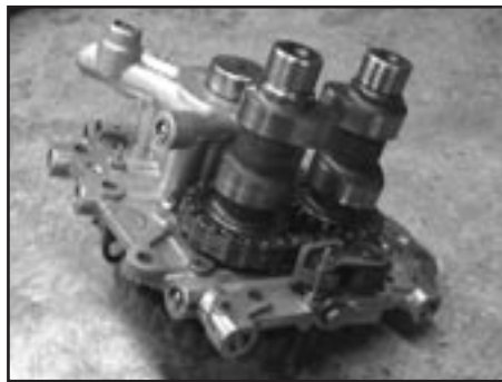
Here is an '03 Road King that just got a 103" Screamin Eagle Kit and is now getting Gear Driven Oil Pump and Cam Assembly
