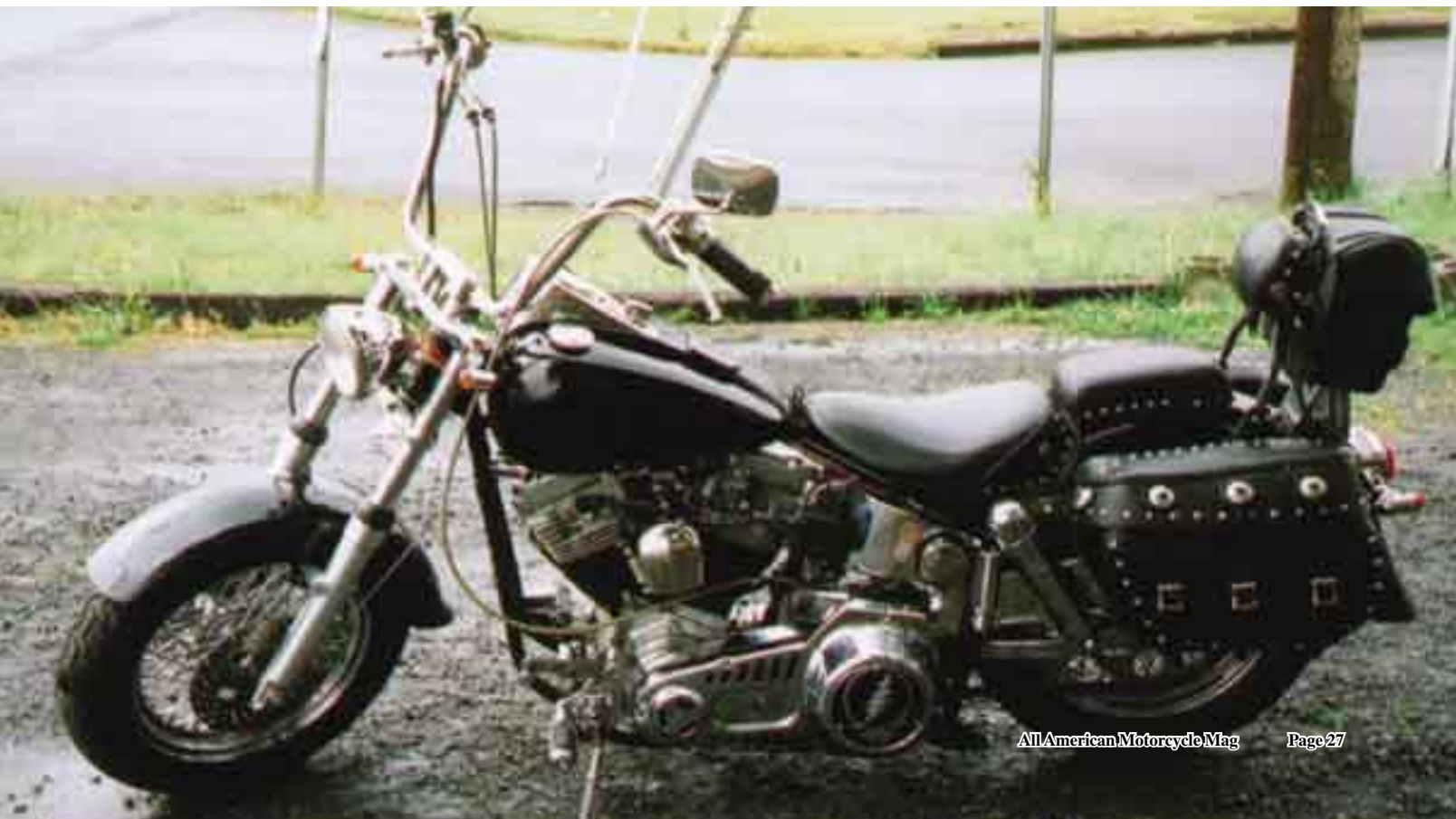
Had to have an Ultima Single fire ignition and coil, chrome saddlebag supports, BDL belt drive, chrome primaries and a custom headlight and Gordon is just about on the road.
